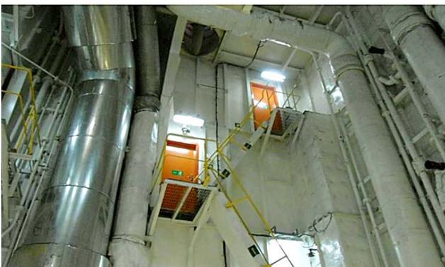
Another point to remember is that some ladders in an engine room lead only to half decks where measurement equipment or gauges are located and these areas may not lead to an escape route – i.e. it is a 'blind alley', therefore mark them as such, with a conspicuous NO EXIT sign.
