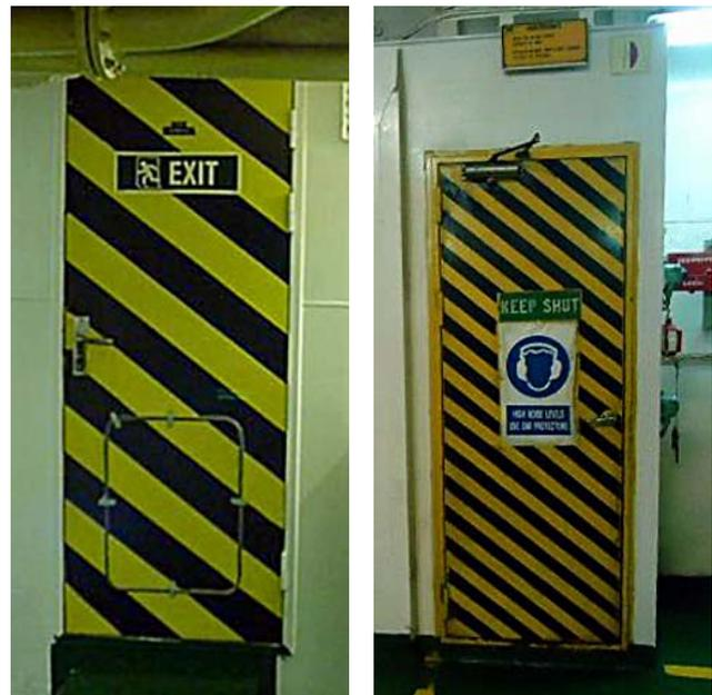
In the event of the engine room being filled with smoke, even light smoke, the escape routes and doors from the engine room may be obscured and therefore they should be more clearly indicated. *You cannot see a white door against a white bulkhead!*
