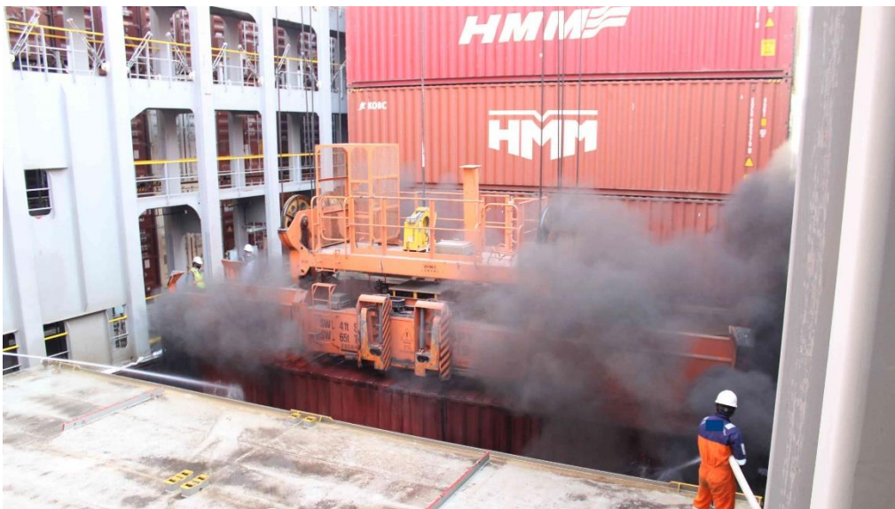
Photograph 5 – Discharge of a container in which there was an ongoing fire amongst a cargo of charcoal tablets.
