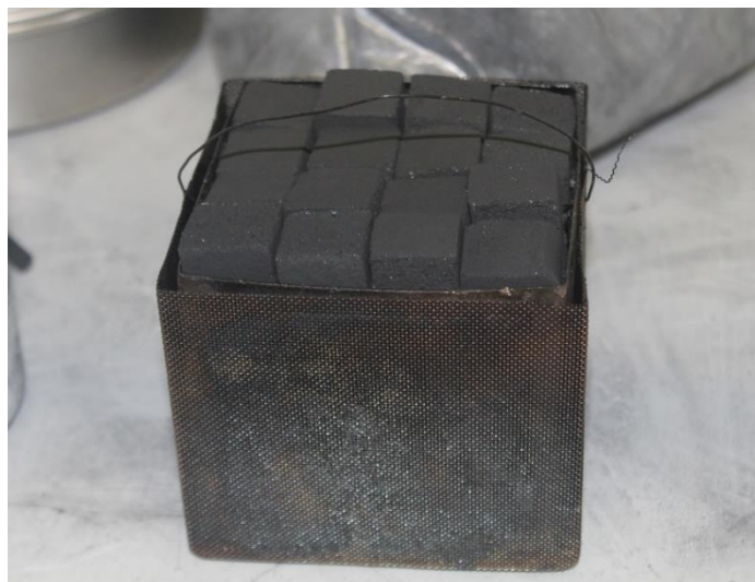
Photograph 4 – Charcoal briquettes arranged in a 100 mm wire mesh cube basket for testing to UN Test N4.
